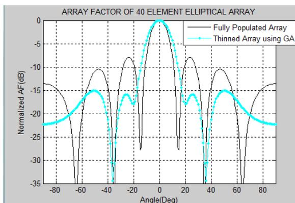
Fig.4. Array factor for 40 element elliptic array
