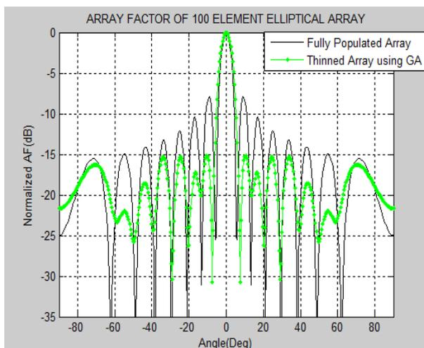
Fig.5. Array factor for 100 element elliptic array
