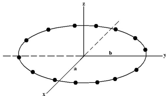
Fig.1. Geometry of elliptical antenna array
