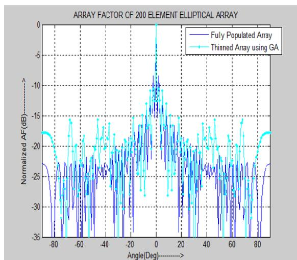
Fig.7. Array factor for 200 element elliptical array
