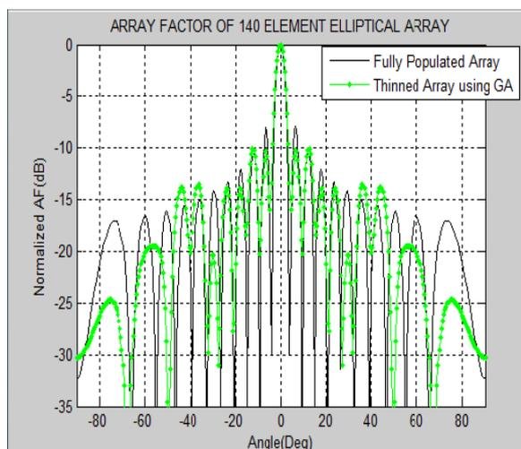
Fig.6. Array factor for 140 element elliptical array
